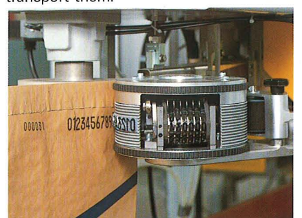
●Imprinter(option) The ink type imprinter is driven by the pinch sealer. Data or numbers are printed on the same position on each bag. A microswitch and a single-rotation clutch are incorporated. Printing types can be changed with ease.
