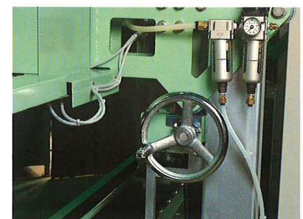
●Machine Height Adjuster Machine height is adjustable simply by turning the handle. The entire sealer rises or lowers, and can be locked at the desired height in a very short time.
